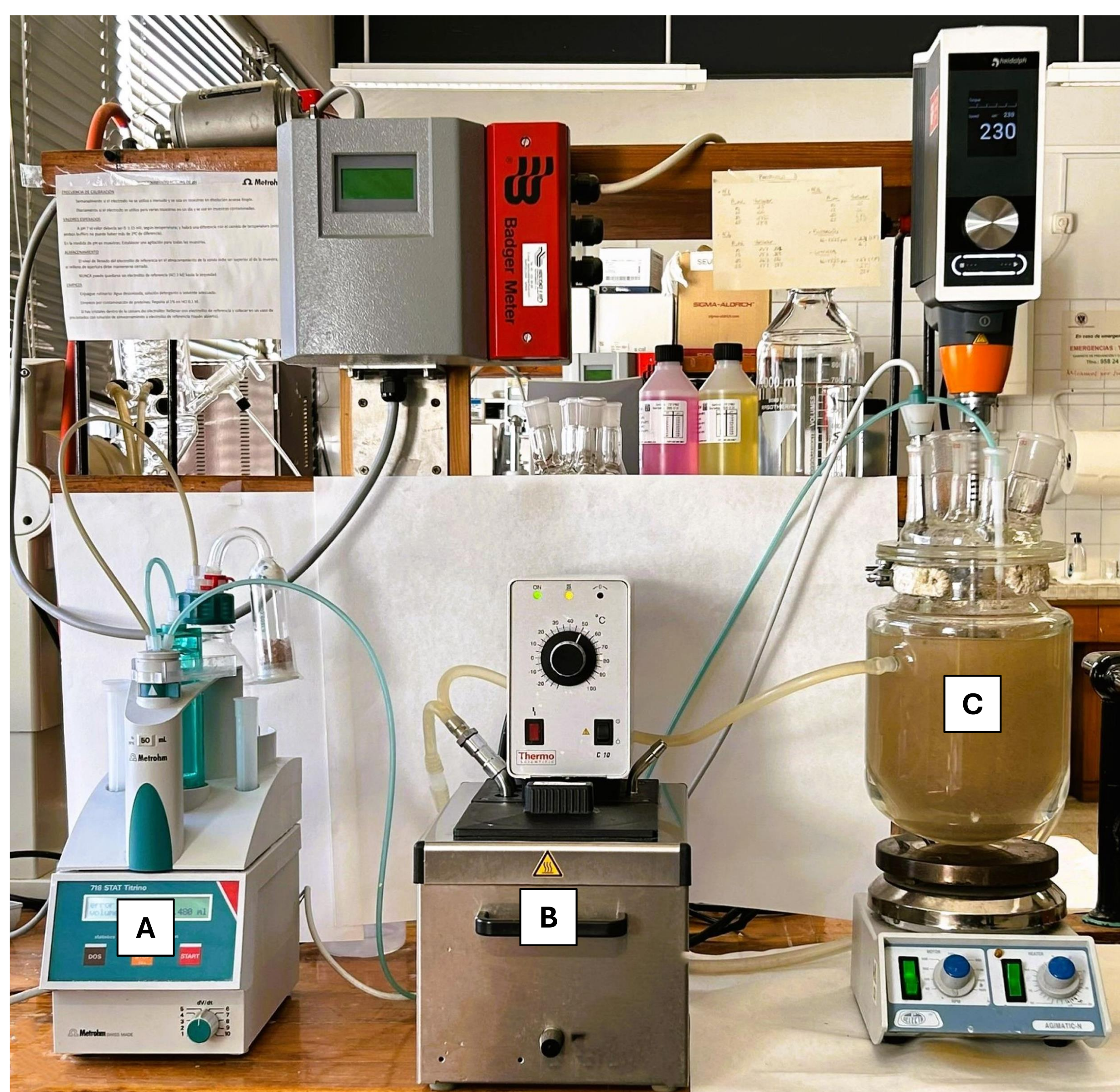
Fig. 1. Experimental set-up. (A) Automatic titrator with pH probe and acid/alkali burette; (B) Water bath; (C) Batch jacketed reactor with mechanical stirring
